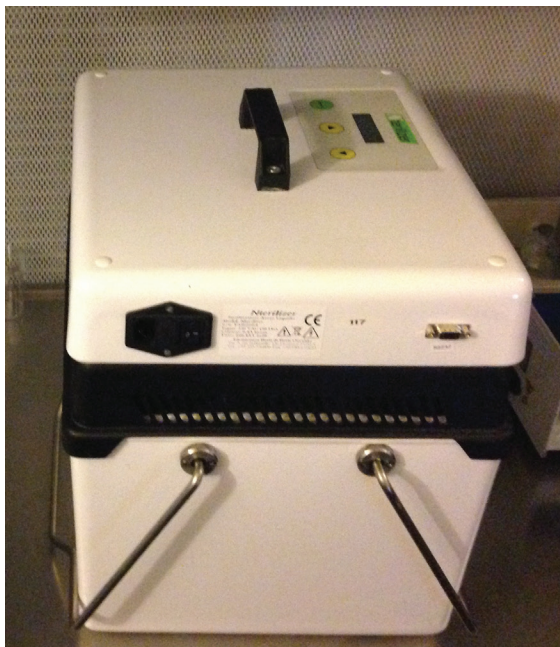
Figure 10.2 Specifically designed device for ultraviolet liquid nitrogen sterilization (Nterilizer— www.nterilizer.com ).
