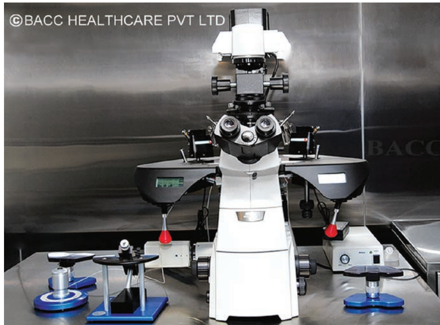
Fig. 2: Inverted microscope with micromanipulator research instrument (RI).
