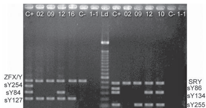
Fig. 12: Electrophoresis on a 1.5% agarose gel showing deletion in the azoospermia factor (AZF) region of the Y chromosome. Ld, molecular weight 100 bp (invitrogen); ZFX/Y, 495 bp; SRY, 472 bp; sY255, 126 bp; sY254, 400 bp; sY134, 301 bp; sY127, 274 bp; sY86, 320 bp; sY84, 326 bp. Lanes 02 and 09, azoospermic patients. Lanes 12 and 16, severe oligozoospermic patients.
