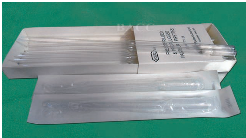
Fig. 19A: Different types of pipettes. (A) Glass Pasteur pipettes and plastic pipettes.
