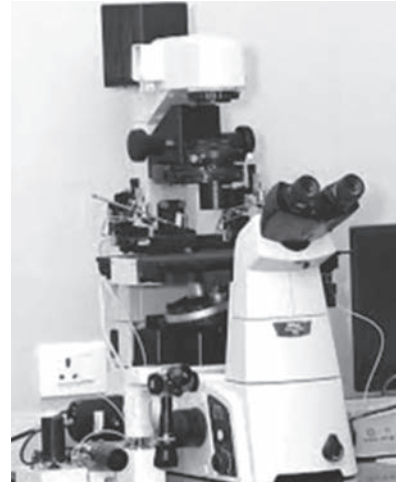
Fig. 11: Micromanipulator with inverted microscope.
