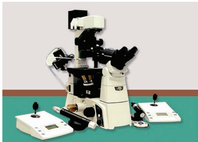
Fig. 8: Eppendorf micromanipulator unit incorporated to Nikon microscope showing motor module unit, control board and oil syringes.
