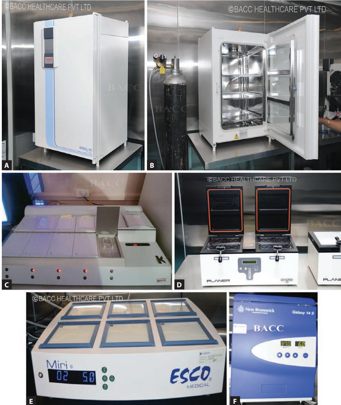
Figs. 3A to F: (A) Box type air jacketed incubator; (B) Box type air jacketed incubator (inside view) with different shelves; (C) Bench top incubator, K systems; (D) Bench top incubator, Origio; (E) Bench top incubator, ESCO; (F) Mini-box type incubator, Eppendorf.
