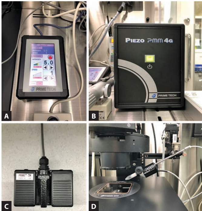
Figs. 11A to D: Four types of equipment of Piezo-ICSI. (A) Operation box; (B) Controller; (C) Footswitch; (D) Drive unit.
