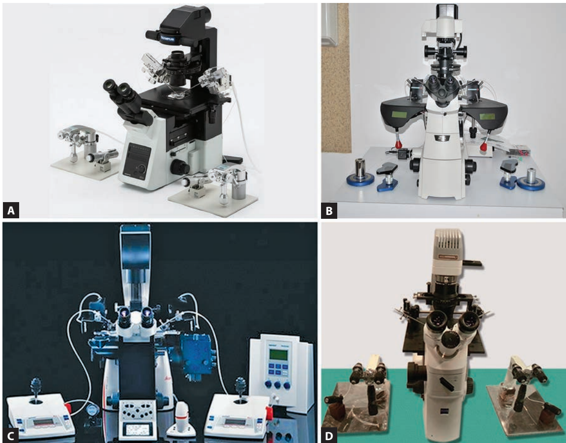
Figs. 2A to D: Different models of intracytoplasmic sperm injection (ICSI) workstations. (A) Olympus inverted microscope with Narishige (Takanome) micromanipulator; (B) Integra workstation (ORIGIO, CooperSurgical); (C) Leica microscope with Eppendorf micromanipulator; (D) Carl Zeiss microscope with S-micromanipulator.
