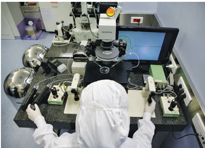
Fig. 1: Two intracytoplasmic sperm injection (ICSI) workstations in opposite direction—a space-saving placement in a busy laboratory. Courtesy: Giles Palmer, Mitera Hospital, Greece.
